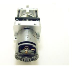
(Note: Motor shown with v1.0 gear selector retainer) Slide the motor into the rear transmission mount, rotating slightly to engage the planetary gears. Push in the motor until the forward case vents are barely flush with the face of the rear transmission mount, as shown. The motor can be installed in any orientation otherwise.
