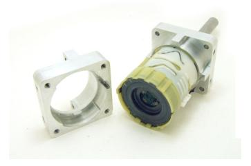
The transmission only fits into the rear transmission mount in one orientation. Line up the notch on the rear transmission mount with the protrusion on the side of the transmission.
