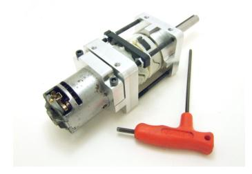
Install the motor clamp ring and the two #10-32 x 1.5" screws using a 5/32" hex wrench. Take care to tighten the screws evenly. When fully tightened, the gap between the motor clamp ring and the transmission mount is approximately 0.025".
