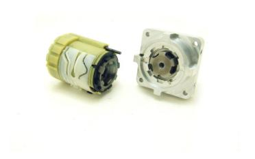
The transmission only fits into the output assembly in one orientation. Use the torque clutch adjustment plunger to align the transmission.
