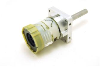
Gently push the transmission into the output assembly while rotating the output shaft with your hand to line up the output spline with the 5-sided output socket.
