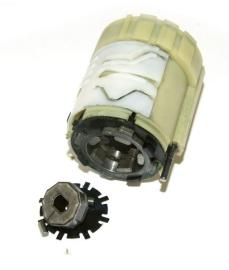
Remove and discard the roller pins, the 5-sided output coupler, and the black steel shim. Reinstall the black plastic cover in the same orientation it was removed from. After this step, the output of the transmission will be a 5-sided socket.
