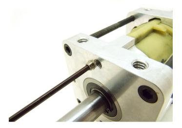
Using a 3/32" hex wrench, screw in the #10-32 x  $\frac{1}{4}$ " set screw into the off-center hole found on the front of the output assembly. As you tighten the screw, the torque clutch plunger will begin moving.
