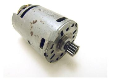
The DeWalt motor has four crimps on the front mounting face which are 1mm larger in diameter than the motor body.
