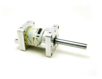
Using gentle pressure, push the rear of the transmission into the mount. Approximately 1/8" of the rear portion of the transmission will be visible.
